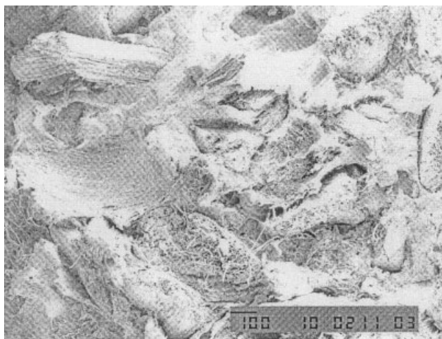
Figure 13 SEM micrograph of a fractured surface of a 30 wt % palm fiber-PP composite with small fibers and no compatibilizer.
