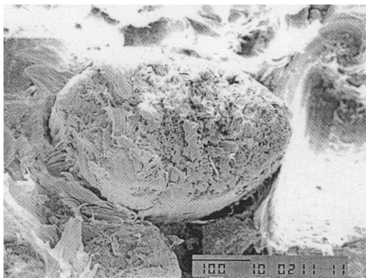
Figure 15 SEM micrograph of a fractured surface of a 30 wt % palm fiber-PP composite (with small fibers) compatibilized with 6 wt % Epolene E-43.
